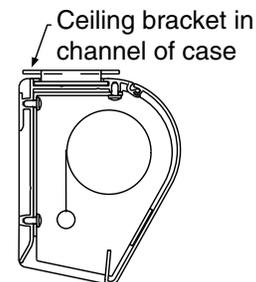
**To mount against ceiling,** hold screen case against ceiling and mark mounting hole locations. Each bracket has 2 holes towards the front edge and 2 holes towards the back edge. Installer must use at least 2 fasteners per bracket with one fastener in one of the two holes closest to back edge of bracket, and one fastener in one of the two hole closest to front edge of bracket. Installer must insure that fasteners are of adequate strength and suitable for the mounting surface chosen.
