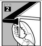
Pinch the ends of the expander with a pliers as shown to hold the black vinyl sweep locked in position.
